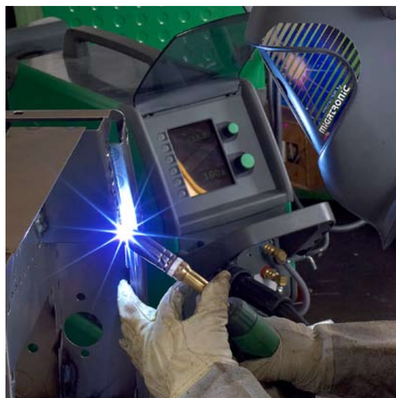
A powerful computer adjusting the process 50,000 times per second is incorporated in the Sigma Galaxy.
